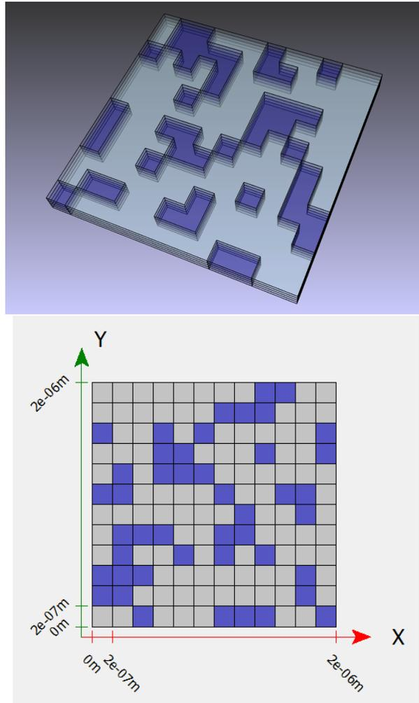
Figure 5: Layer Stackup View After Optimization(top), Pattern View (Bottom)
